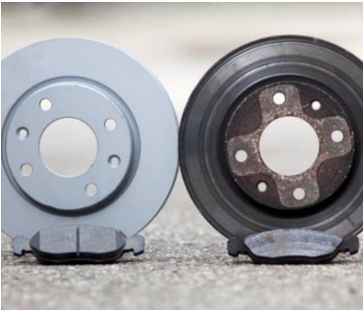
Fig.1 Worn rotor & Pad comparison
